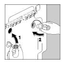
You can now see the openings that must be closed with the caches in the pack attached to the washing machine; do not forget to fold down the central capsule.
